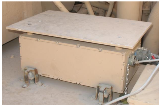
Fig. 2: ARMY eDAQ TWV Package with lid removed
