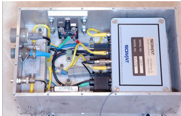
Fig. 2: ARMY eDAQ TWV Package with lid removed
