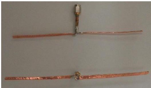
Fig 3: Constructed dipoles
