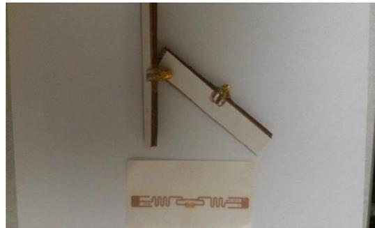
Fig 4: Prepared Alien 9640 Squiggle Inlay RFID tag
