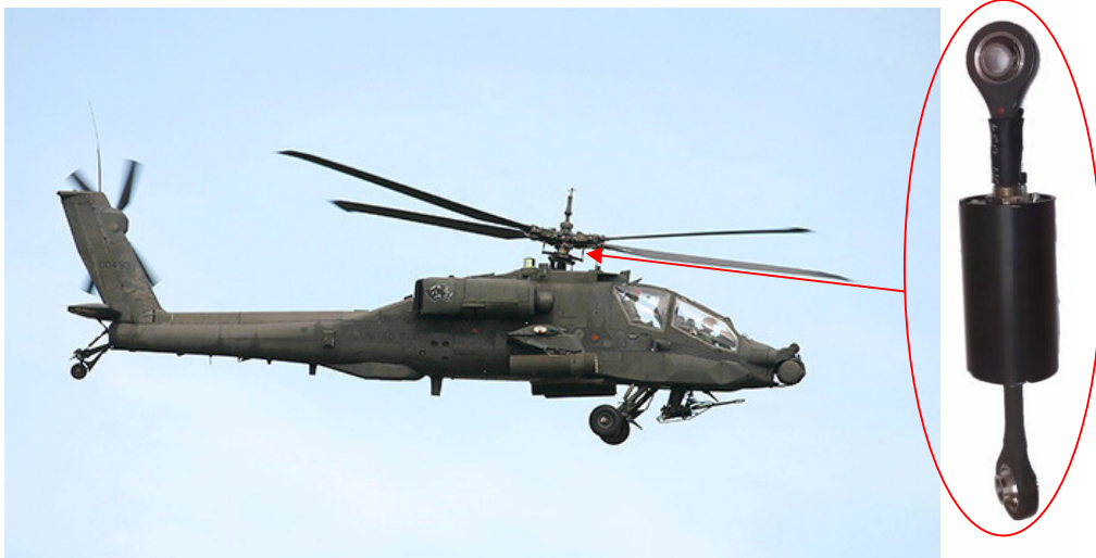
Figure 3: Apache Pitch Link Energy Harvester and Sensor Node.
