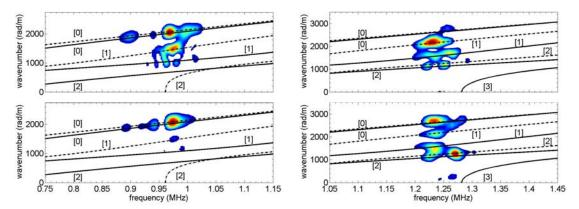
Fig. 8: Spectral decomposition of wave field acquired using FBG sensor array at 950 kHz (left) and 1.25 MHz (right). The top figures show the results for the plate in pristine condition and the bottom figures for the plate with a notch.
