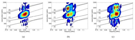
*Fig. 7: Spectral decomposition based on a low spatial resolution of the wave field at 950 kHz for (a) pristine plate; (b) a 14 mm long, 1 mm deep notch and (c) a 14 mm long, 2.5 mm deep notch.*
