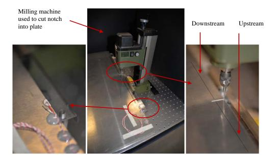
*Fig. 1: Experimental set-up showing the semi-circular piezoelectric source element (left); the milling machine to create the notch (middle); and the tungsten carbide miller (right).*
