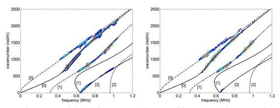
Fig. 2: Upstream (left) and downstream (right) spectral decomposition for pristine plate. Dotted lines denote dispersions lines for antisymmetric modes and solid lines for symmetric modes. The modal order is given in parentheses.
