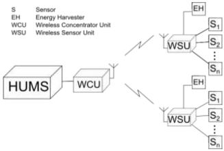
Fig. 1: Honeywell HUMS wireless architecture
