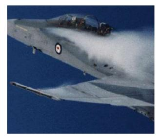
*Fig. 2: Vortices shed from the leading edge extension of the wing causing buffeting over the empennage*
