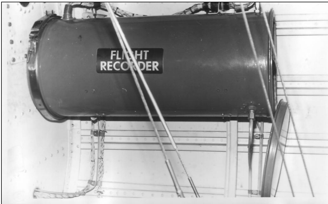
Figure 3: The canister in the tail containing the FDR
