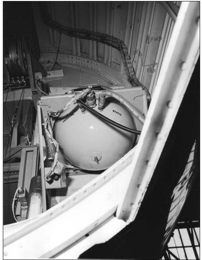
Figure 5: Lockheed Aircraft Service model LAS-109C FDR
