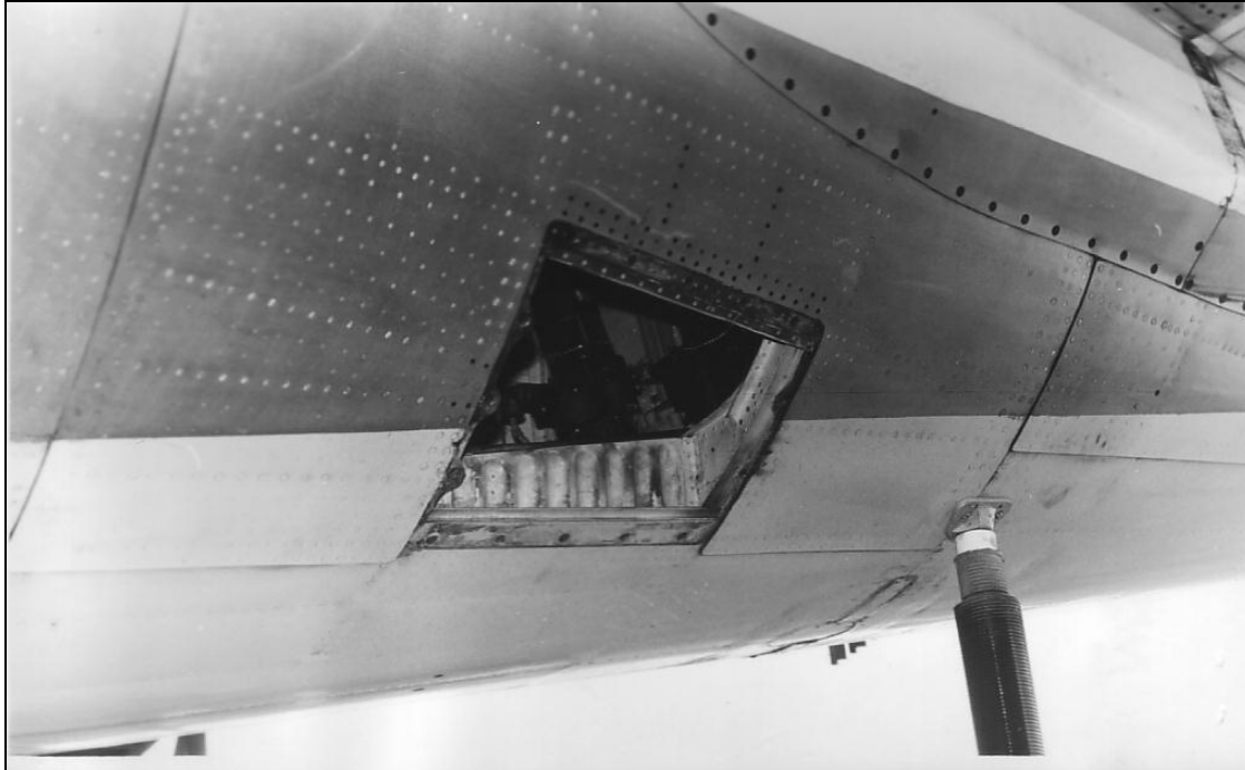
Figure 2: Access to FDR via access panel in rear fuselage
