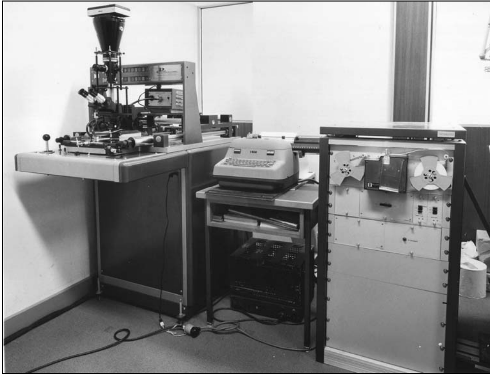
Figure 18: Early Australian readout equipment for analogue FDR's
