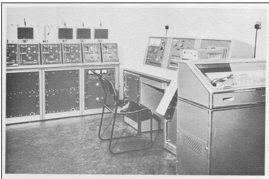
Figure 19: An early UK readout station for digital FDR's 27
