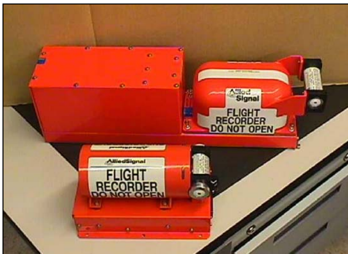
Figure 1: Developments in solid-state FDR's show a decrease in size and weight 7
