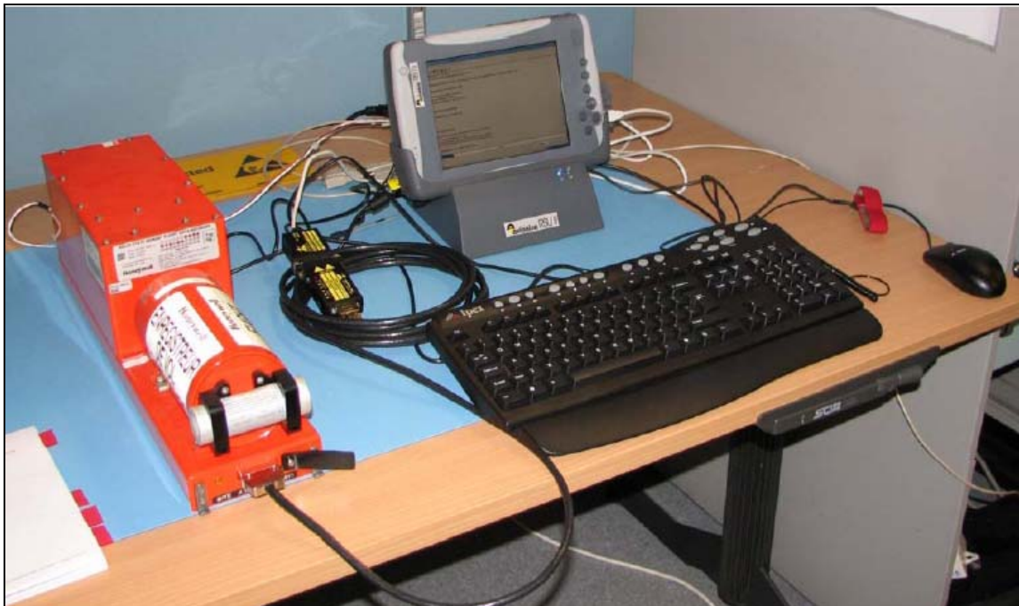
Figure 15: Downloading data from a solid-state FDR
