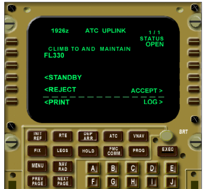
Figure 11: Example presentation of a datalink message on a cockpit MCDU 20
