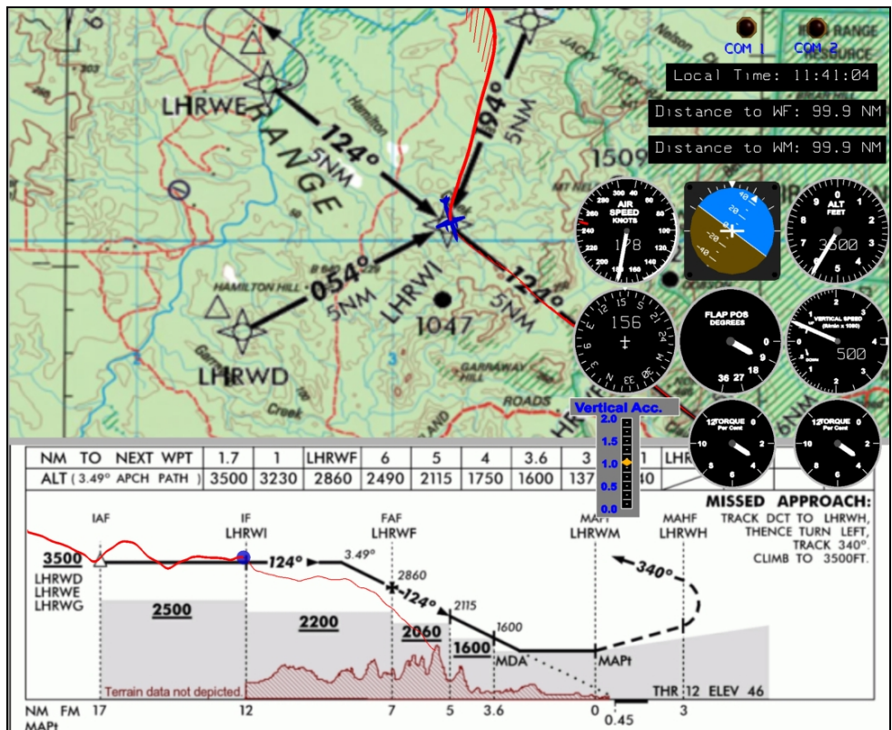
Figure 25: Animation showing plan and elevation views of an instrument approach 34
