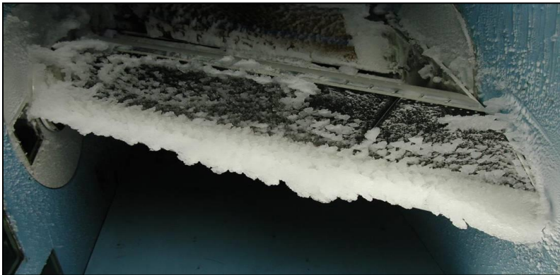
Ice buildup after 45 min hold
