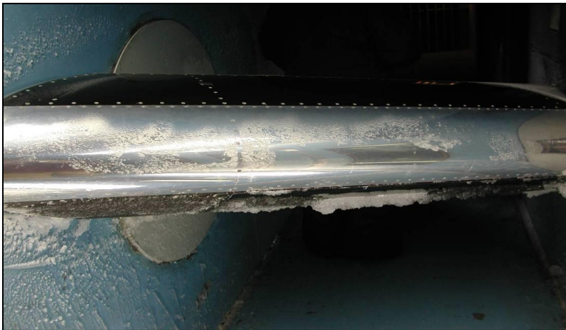
Actuator removes 5" glaze ice pack
