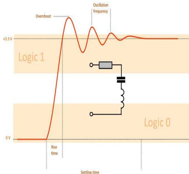
**Figure 6** A digital line switching from logic level 0 to 1 might act as shown. If the system is underdamped as a result of high capacitance, the rise time can be very high with no overshoot. The ideal is the critically-damped response that minimises overshoot and settling time [10].
