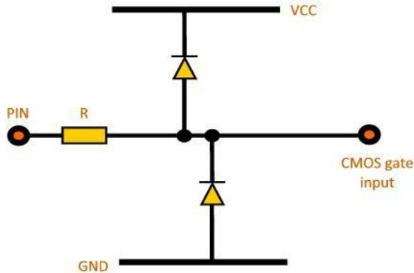
**Figure 4** CMOS logic gates include overvoltage clamp diodes as shown.
