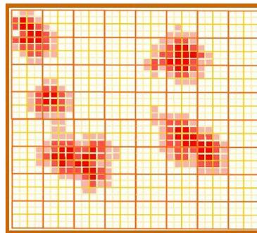
**Figure 10** This SOFM map has 1024 neurons (32 x 32) and the clustering suggests 4/5 distinct modes of operation for the system. In the test phase following training, a test vector finding the closest neuron to be away from the clusters could be the indication of a fault condition (or merely the system being used in a new way that did not occur during training).
