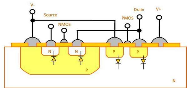
**Figure 5** At die level diodes exist when the device is unpowered.
