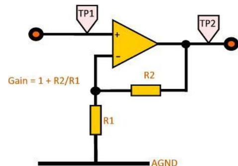
**Figure 7** The action of the operational amplifier and the two resistors can be derived from the voltages on test points 1 and 2
