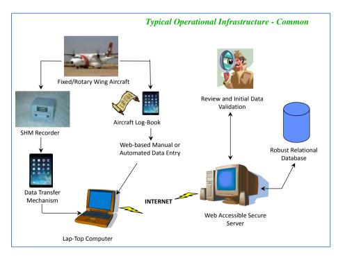
Figure 5: Typical Operational Data Acquisition and Validation Infrastructure
