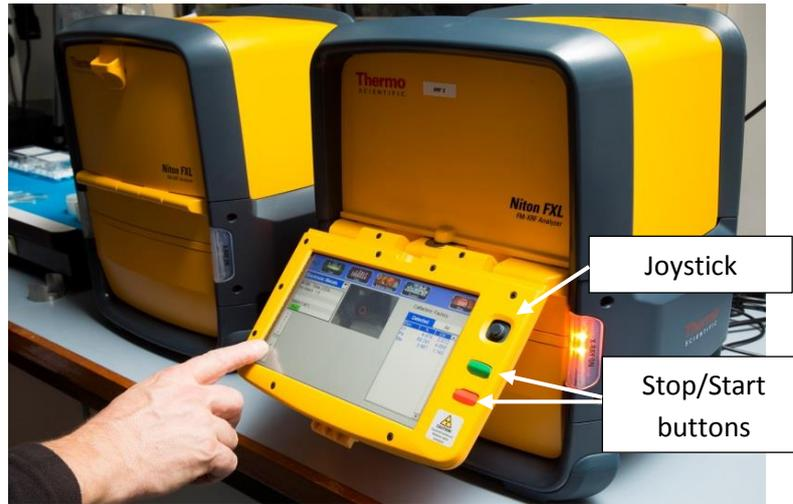
Figure 5: Niton FXL XRF Overview
