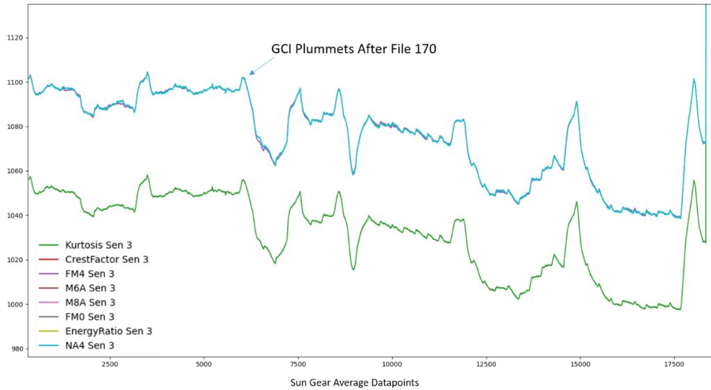
Figure 3: Channel RL-3 (Sensor 3) Kurtosis, NA4, and FM4 Gear Condition Indicators with 10 sun gear revolution rolling average.
