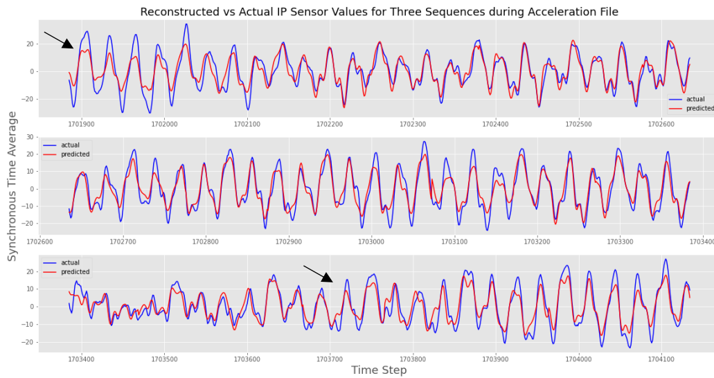
Figure 4. Example reconstruction at the acceleration point for the VS-LOO algorithm showing significant reconstruction amplitude degradation at low and high frequencies with consistent under-prediction.
