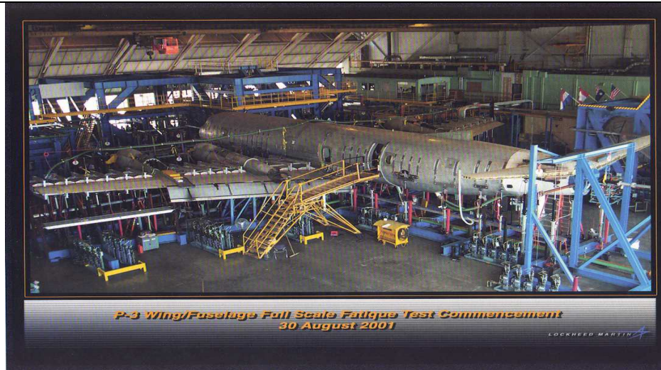
Figure 2: USN P-3C Wing/Fuselage Full Scale Fatigue Test Article at Lockheed Martin
