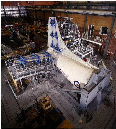
Figure 3: DSTO P-3C Empennage Full Scale Fatigue Test
