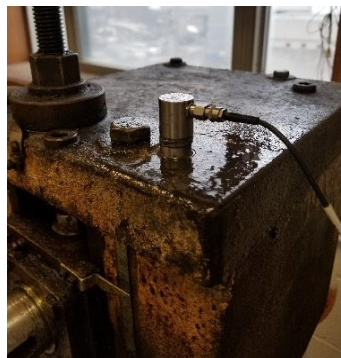
Figure 2. Sensor installed at the gearbox housing top
