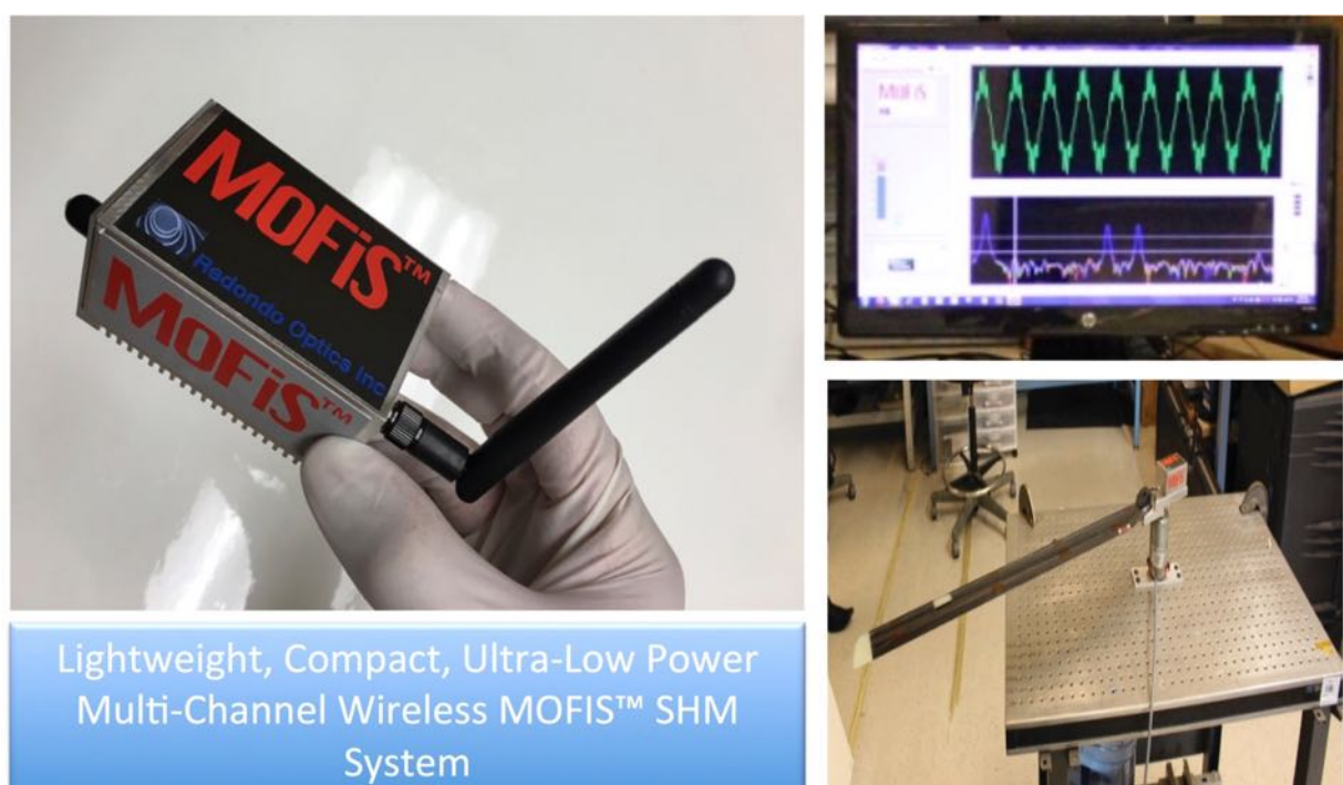
Fig. 4: Performance Testing of MOFIS™ System on a 1-meter Long Simulated Downscale Helicopter Composite Blade.
