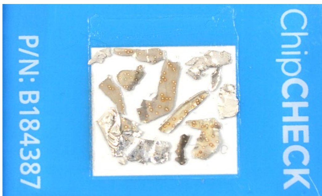
Figure 1: Sample of silver (Ag) plating showing where the laser has ablated the surface during analysis in the ChipCHECK.
