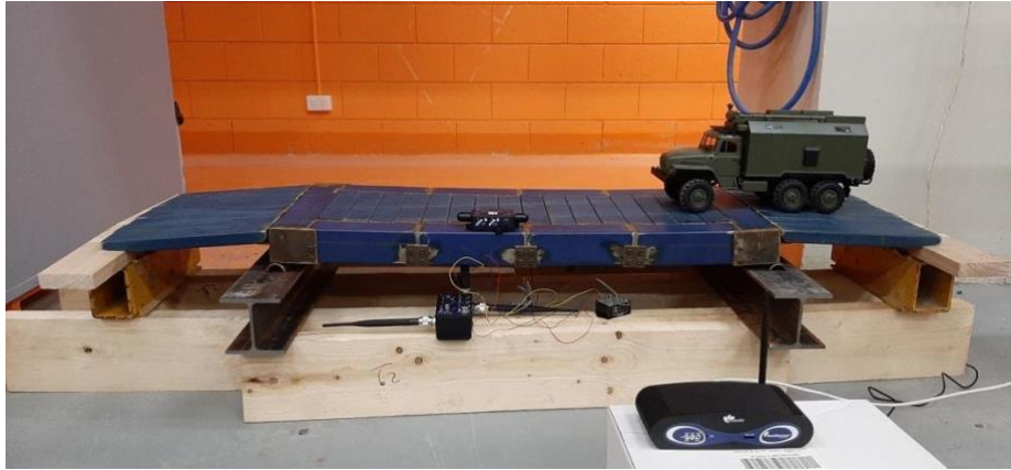
Figure 1: The lab-scale modular bridge and the wireless sensing system
