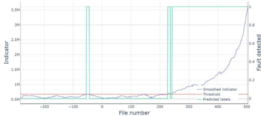
Figure 4: The proposed indicator and threshold using FRESH filters on the full dataset up to file 500 of the original dataset. Final files not plotted due to large exponential increase.
