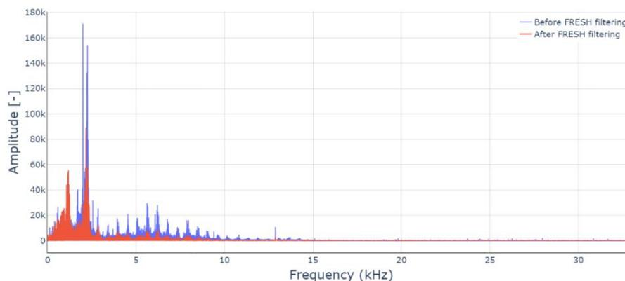
Figure 1: Frequency representation of a signal with a severely progressed fault (file 522 of the original dataset). Sensor located on the rear of the ring gear.
