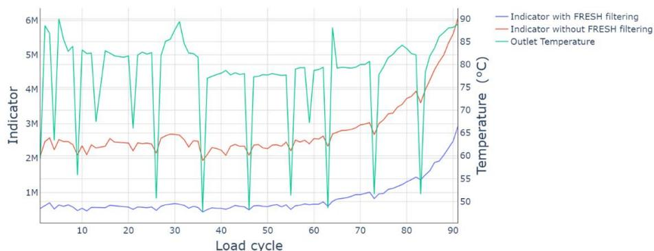
Figure 3: The proposed indicators averaged per load cycle and outlet temperature over the full dataset. Last load cycles not shown due to exponential increase.
