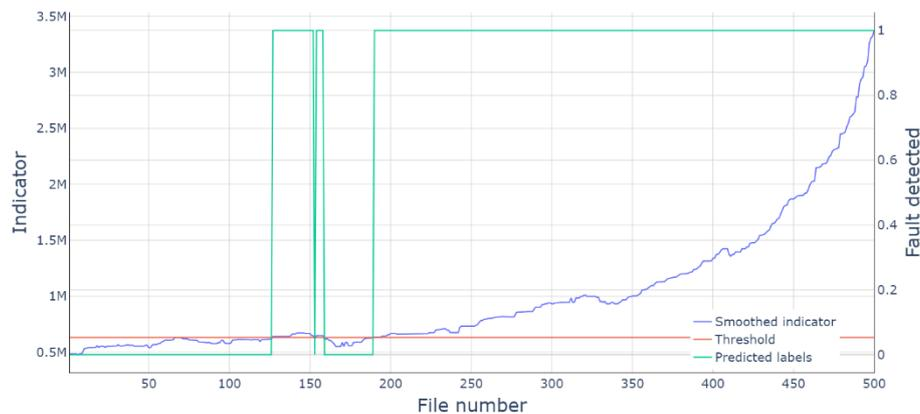
Figure 2: The proposed indicator and threshold using FRESH filters on the original dataset up to file 500. Final files not plotted due to large exponential increase.
