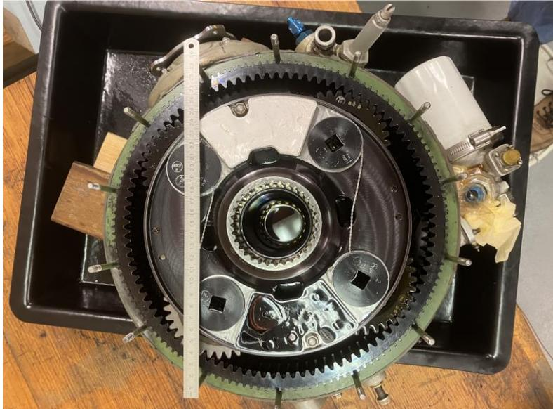
Fig. 3: Sensor and balance weight mounted on planet gear carrier.
