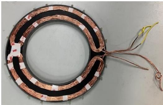
*Fig. 1a: WPT coils in carrier*
