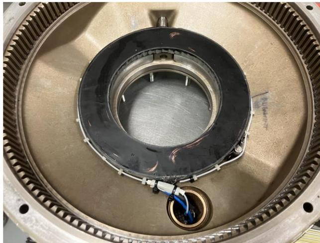
*Fig. 2: WPT coil and RF receiver antenna mounted on gearbox housing*
