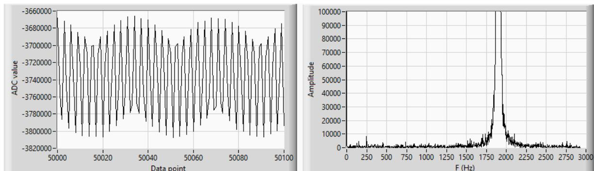
Fig. 4: Shaker test at 1.9kHz and 1G acceleration, time domain waveform(left) and frequency spectrum (2048 samples) on right.
