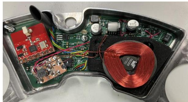
*Fig. 1b: Sensor assembly prior to potting*
