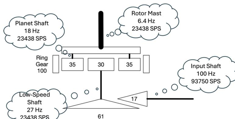
Figure 2 Notional Gearbox using Global Tach-from-Vibration Processing.
