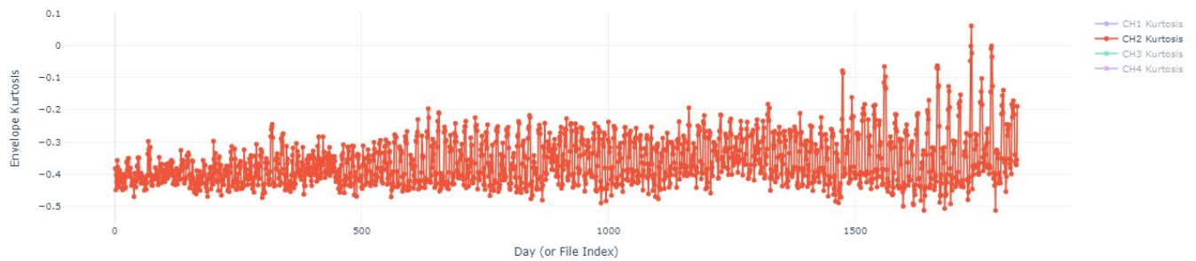
Figure 5: Envelope Kurtosis trend over time for the 2 nd channel (sensor nearest to the crack location), using data from all three torque ratings: 100%, 125%, and 150%.
